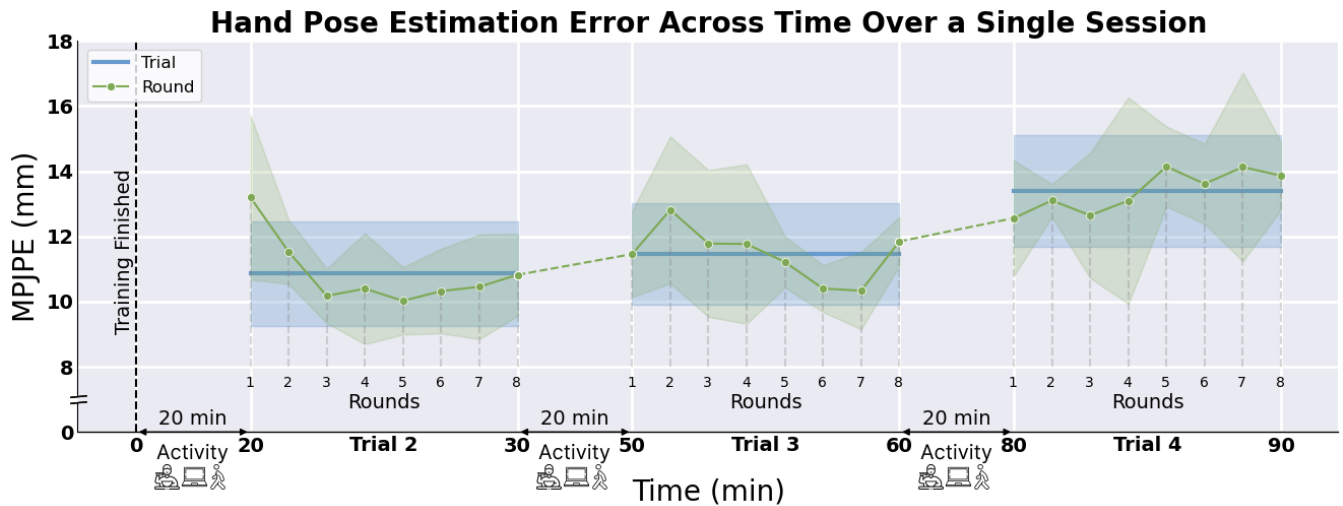
Figure 4: EITPose mean per-joint positional error (MPJPE) averaged over participants across time for a longitudinal session. Filled Areas/Error bars indicate standard deviation.
