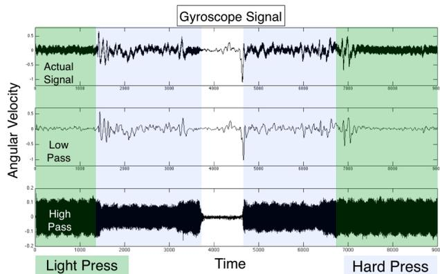
**Figure 3. (top)** Gyroscope signal when user presses light, then hard, then waits for a second and presses hard and soft again. **(middle)** The lower frequencies generated from touch-induced vibrations *increase* with increase in pressure. **(bottom)** Motor-induced vibrations are diminished as the amount of pressure exerted increases.
