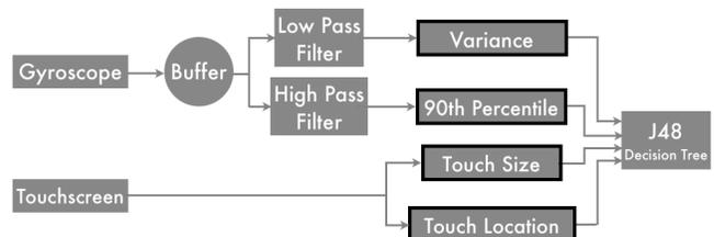
**Figure 4.** Block diagram of the major components of GripSense’s pressure detection module. Low frequency variance, 90<sup>th</sup> percentile of higher frequencies, touch size and location are the features used for classification.
