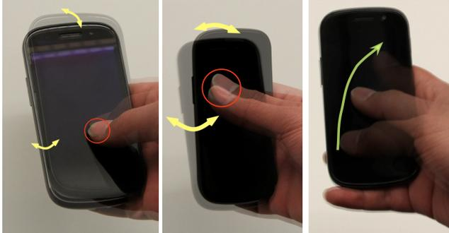
**Figure 2.** (left) Minimal device rotation in  $x$ - and  $y$ -axis, and smaller touch size when the user touches nearby with the thumb. (center) Significantly more rotation in  $x$ - and  $y$ -axis and larger touch size when the far quadrant of the screen is touched. (right) The shape of the swipe arc in the case of right thumb. (All of these phenomena are mirror-imaged for the left thumb.)
