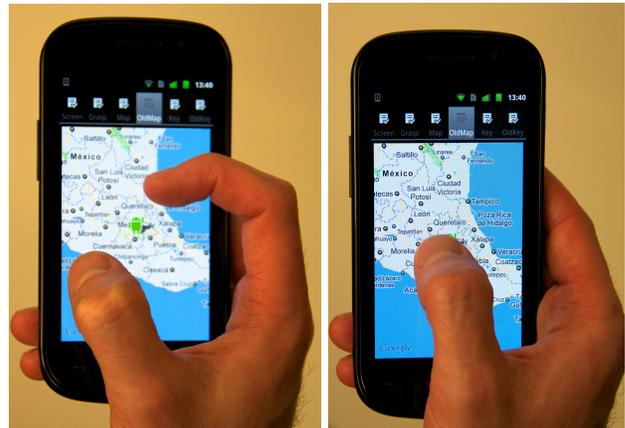
**Figure 1.** (left) It is difficult for a user to perform interactions like *pinch-to-zoom* with one hand. (right) *GripSense* senses user’s hand posture and infers pressure exerted on the screen to facilitate new interactions like zoom-in and zoom-out.
