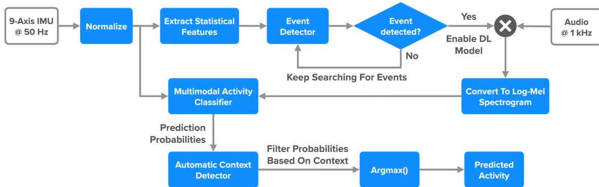
Fig. 3. Overview of SAMoSA's System Architecture.
