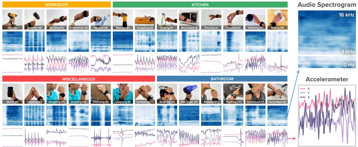
Fig. 2. SAMoSA is a human activity recognition system that uses IMU motion data sampled at 50 Hz and sound sampled at  $\leq 1$  kHz. The figure showcases the 26 different activities (with associated contexts) that our system can recognize, along with sound spectrograms (log scale, with 1 KHz cutoff denoted with a solid white line) and 3-Axis accelerometer streams.
