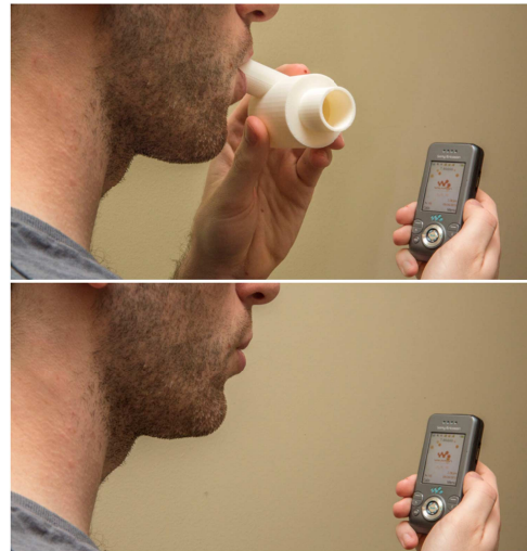
Figure 1. A user using SpiroCall on a feature phone (Sony w580i) with, and without a SpiroCall whistle.
