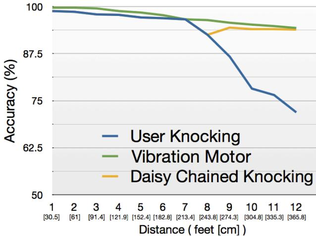
**Figure 7.** Performance of detecting devices on the same surface. User knocking performance drops significantly over larger distances, but this can be nullified using daisy chaining.
