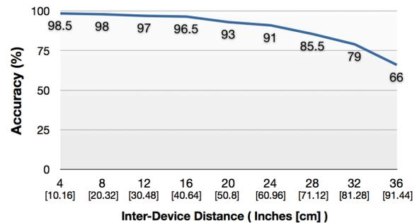
Figure 11. Performance of acoustic stereo positioning.
