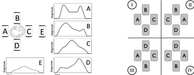
**Figure 6.** (Left) The timestamp of the audio peak for each device informs the order of devices. (Right) Four possible arrangements of devices.
