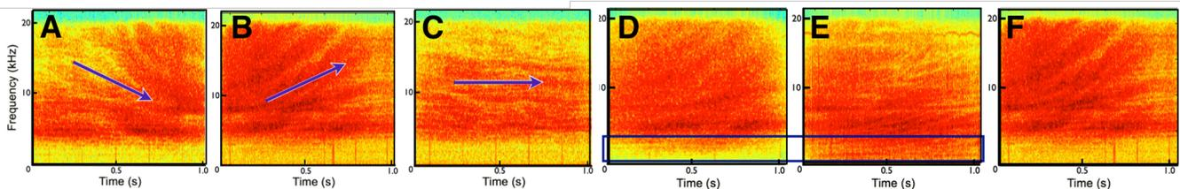
**Figure 3** (A) Swipe towards the device. (B) Swipe away the device. (C) Vibrations experienced by the non-participating device. (D) Gesture performed with fingertip. (E) Gesture performed with fingernail. (F) Gesture performed with fist
