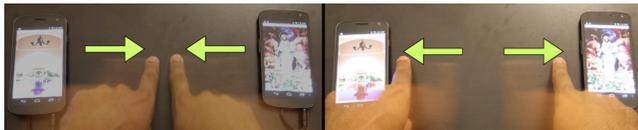
Figure 4. (Left) Pinch gesture, (Right) Expand gesture
