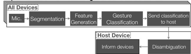
Figure 5. Block diagram of major components of SurfaceLink's gesture detection. Pattern matching results from all devices are sent to the host device for disambiguation.
