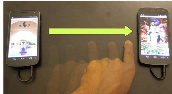
**Figure 1.** User interacting with two mobile devices on a shared table using only on-device inertial and acoustic infrastructure and inexpensive contact microphones.
