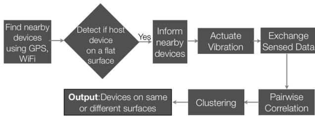
**Figure 2.** Block diagram of major components of SurfaceLink’s detection of devices on the same surface. When sensing user-induced vibrations, inertial sensor data is used, and when sensing device-induced vibrations, the contact microphone data is used.
