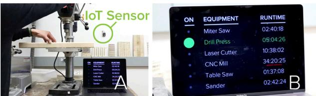
**Figure 18. Sound-driven IoT sensors could track equipment use (A) for safety and maintenance (B).**
