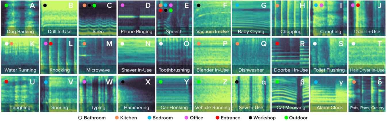
Figure 7. Example log Mel spectrograms (based on [16]) of 960ms audio for our 30 test event classes. These  $96 \times 64$  input vectors are used to tune a VGG-16 model pre-trained on YouTube-8M.
